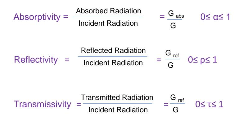
**IRRADIATION, G:** Radiation flux incident on a surface is called irradiation.
